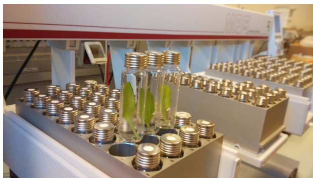
Fig. 1 Autosampler used for leaf screening. Vials with single Arabidopsis leaves in the autosampler blocks
