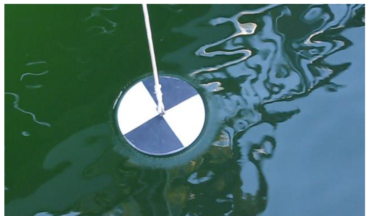
A Secchi Disk. (Credit: Lakes of Missouri Volunteer Program / University of Missouri)
