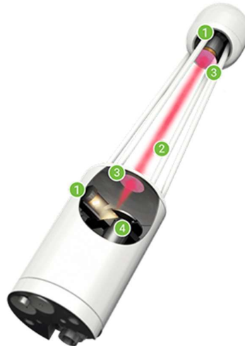
Figure 2-3 Drawing of the LI7550Rs, Open path InfraRed Gas Analyser. 1) Laser source and detector 2) open path with laser beam 3) scratch-resistant lenses 4) chopper motor and chopper wheel. (source: http://www.licor.com/ )
