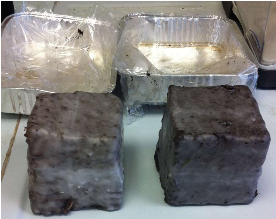
Figure 3-6 Two cubes of paraffin covered peat blocks of 10*10*10 cm used for the measurement of hydraulic conductivity.
