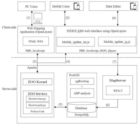
Figure 1: Architecture of routing as web services
