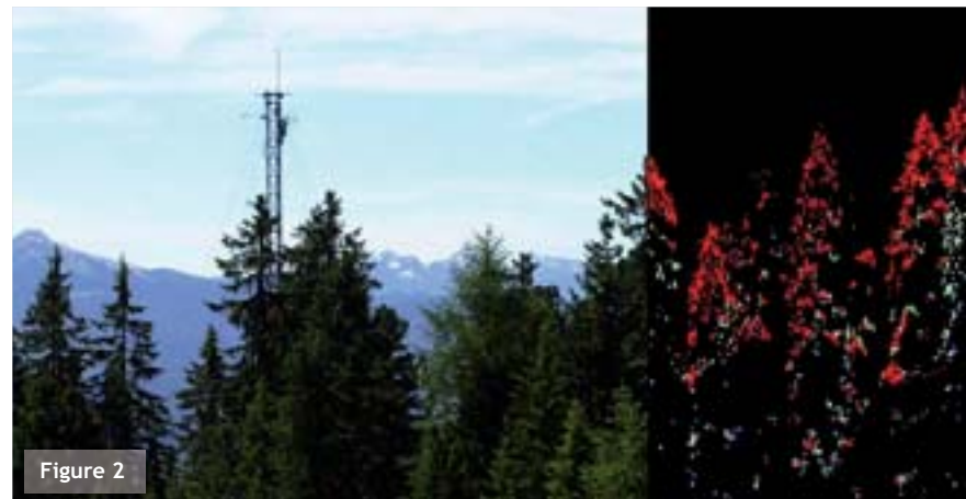
Fig. 2 - Multiple returns Light Detection and Ranging (LIDAR) data of a coniferous forest
