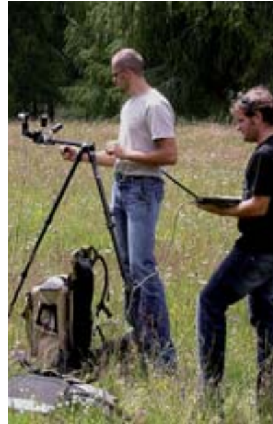
Fig. 4 - Spectroradiometric measurements campaign to obtain high spectral resolution vegetation reflectance data
