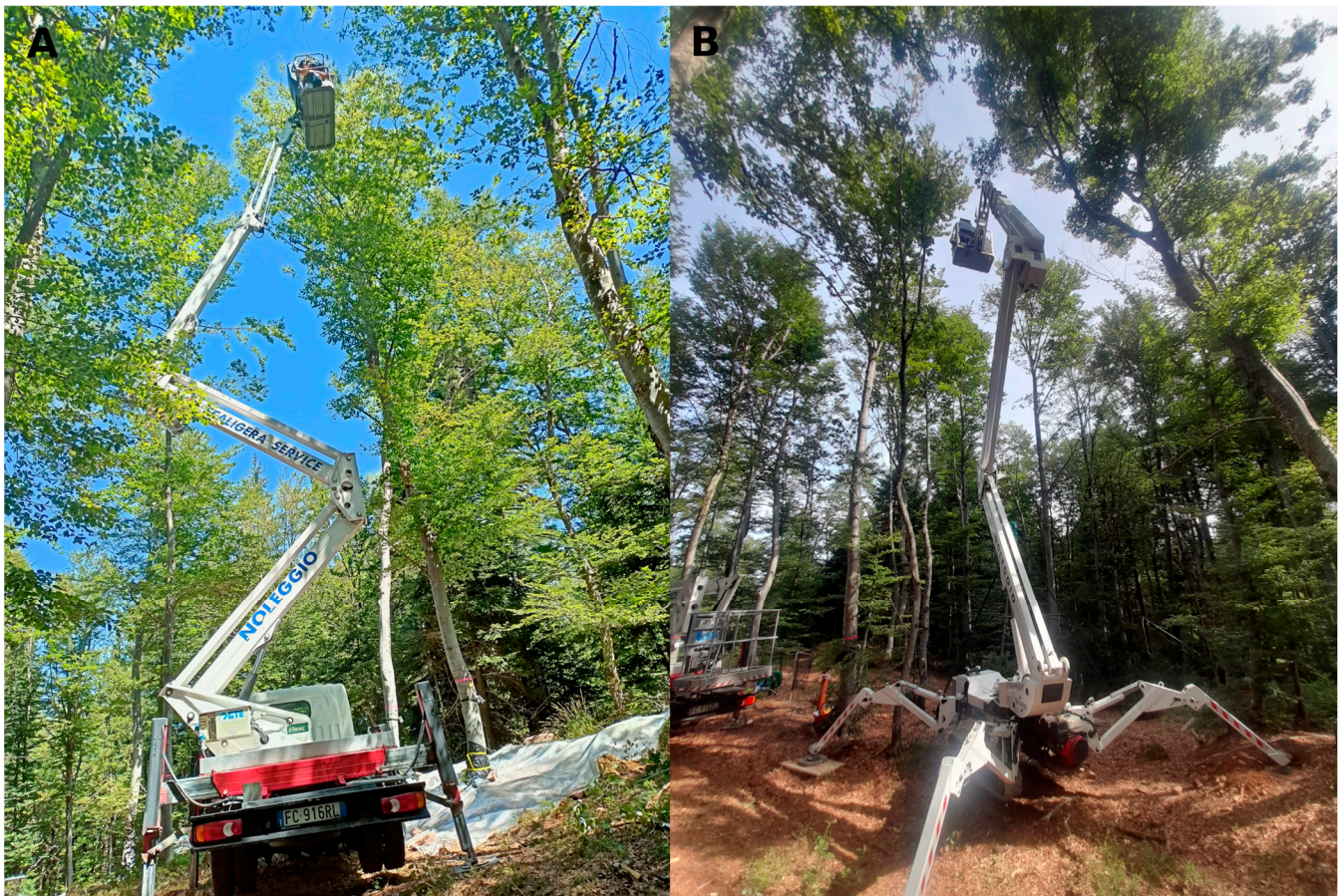
Figure 1. The two mobile elevating work platforms used for ecophysiological measurements: the truck-mounted lift (A) and the spider lift (B).
