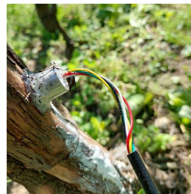
Fig.6 Stem Water Potential probe by FloraPulse Co. (Lakso et. al. 2002)
