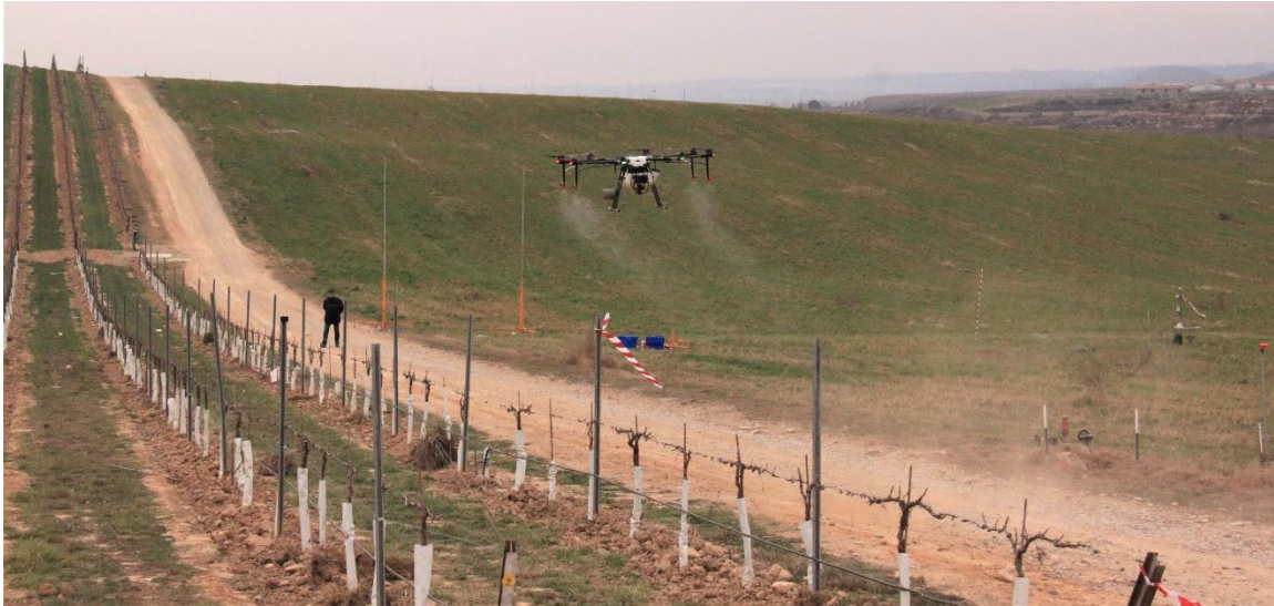
Fig. 1. Aerial and sedimenting drift test in a vineyard in wintertime.
