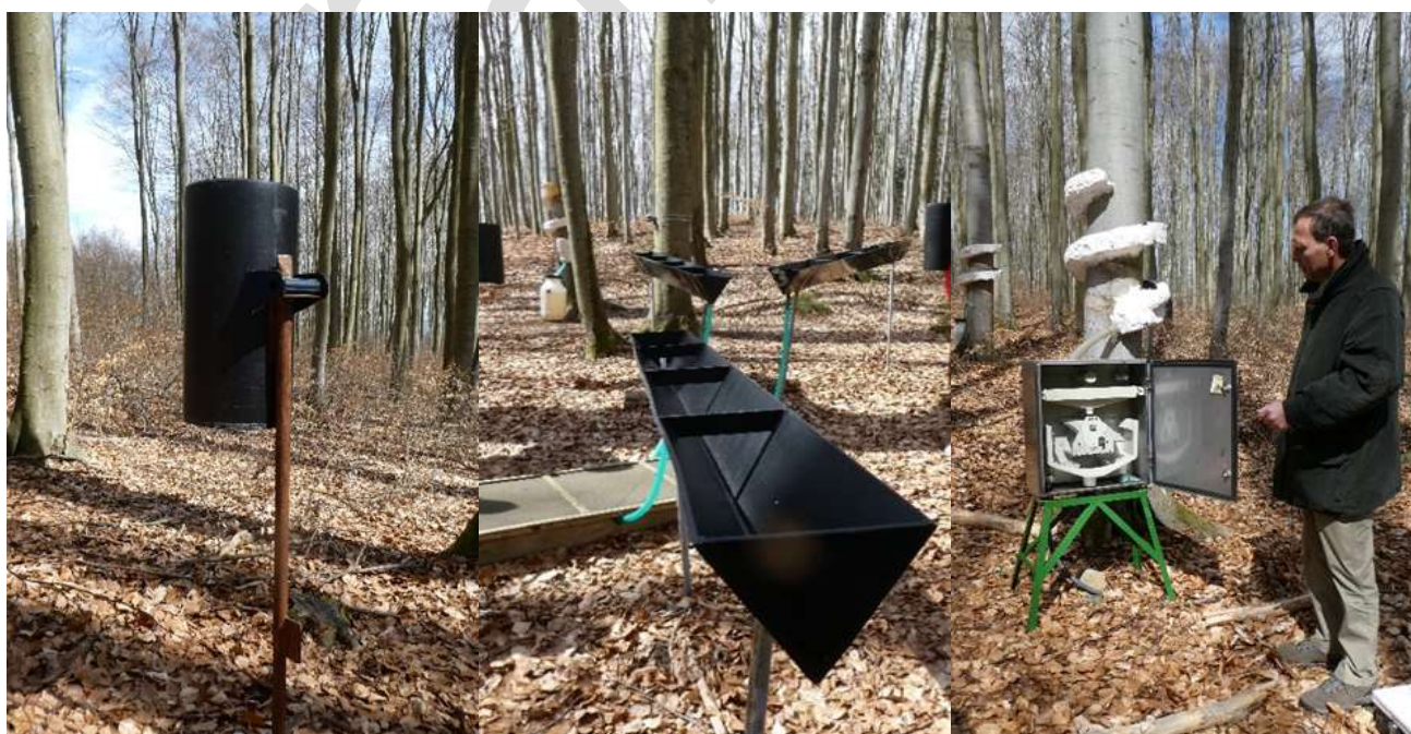
Figure 6.1: Snow sampler (left), rain sampler (middle), and stemflow sampler (right) to determine throughfall deposition at an ICP Forests Level II site in south-western Czechia (Images: Peter Waldner)
