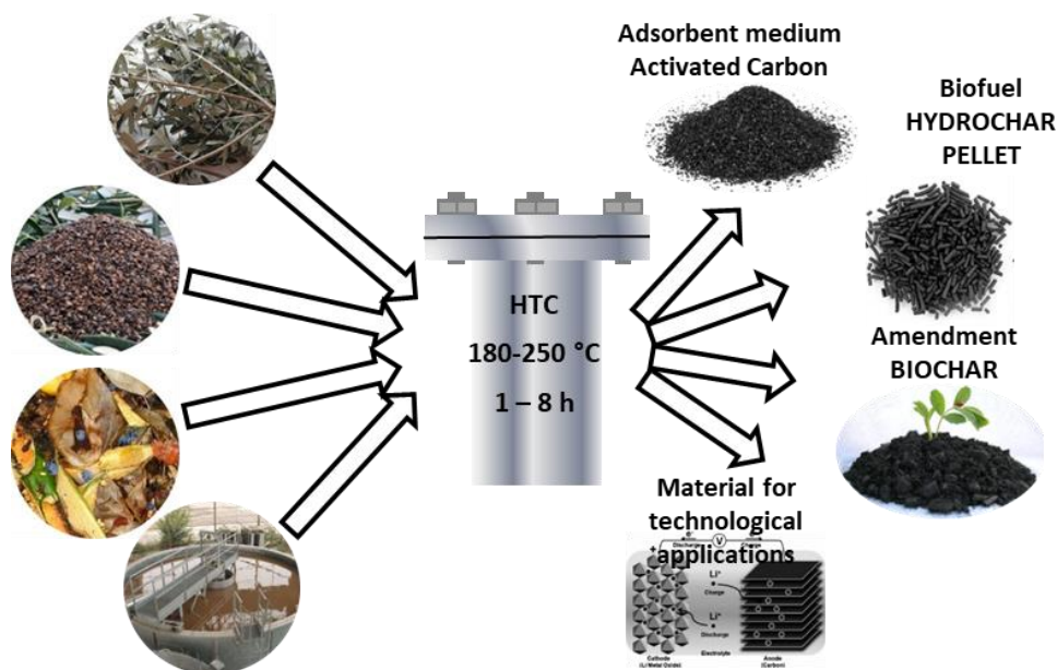
Fig. 1 - An indicative scheme of different biomass types suitable for HTC and possible HTC solid products
