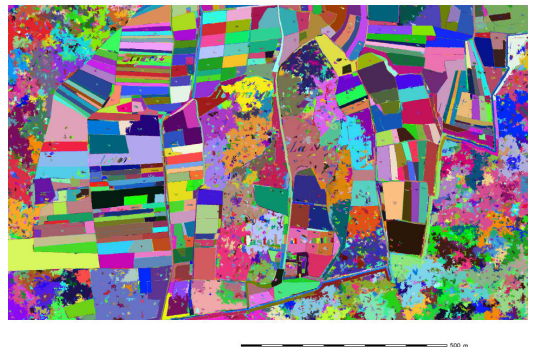
Figure 5. Segments for threshold value of 0.1 and minimum number of cells in a segment of 25 - particular.
