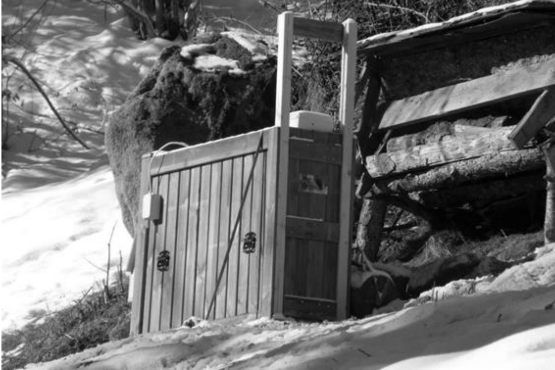
Figure 1 Box trap used for capturing roe deer. To note on the front side (i.e. the one close to the door that is shown in the image) the white box containing the modem to remotely alert the capture team.
