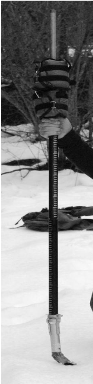
Figure S1.2 The whole penetrometer calibrated for this study (left) and the particular of the tip of the penetrometer (right).
